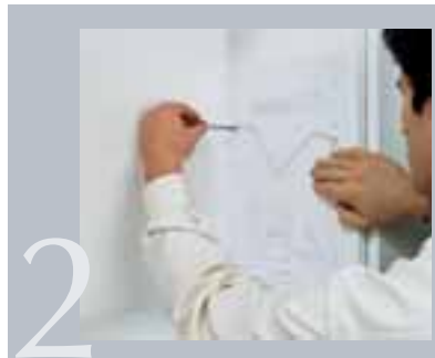
2 MARK WITH A PUNCH TOOL AS INDICATED ON THE TEMPLATE. VARIOUS OPTIONS ARE AVAILABLE, DEPENDING ON THE DESIRED ANGLE OF THE PLATE-RACK. CARRY OUT STEPS 1 AND 2 ON BOTH SIDES OF THE UNIT.
